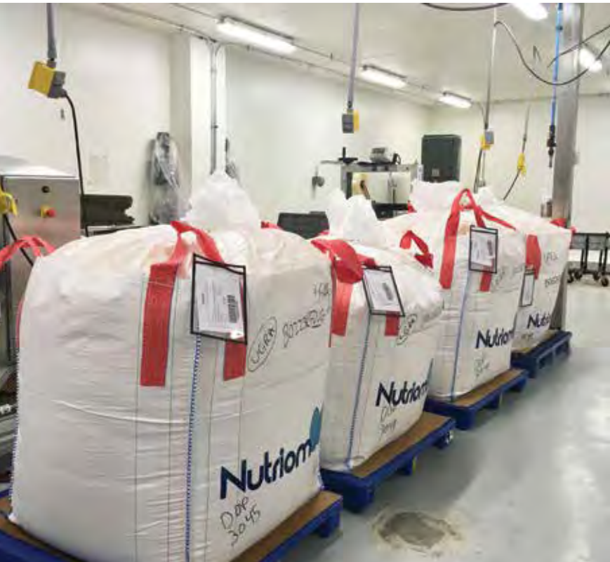
These 1,000-pound bags are filled with egg powder that came from the slow drying process used by Nutriom. The next step is to freeze dry the powder to create the egg crystals the company sells in a variety of products.
