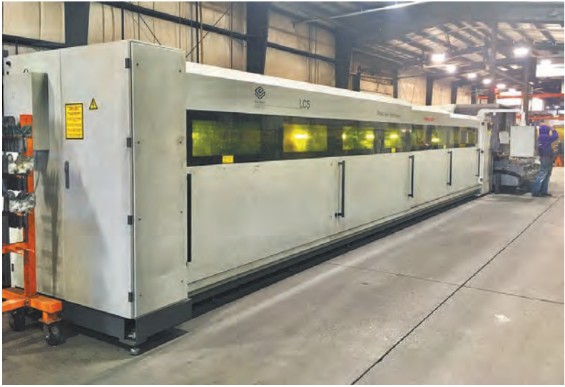
This laser in the Power Lift manufacturing facility is used to cut holes in metal pieces of equipment. Metal signage the company offers to customers to fit on the equipment they purchase also is created on this machine.
