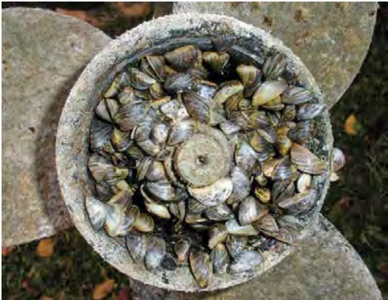
This boat prop clogged with zebra mussels is an example of what could happen at Lake Panorama if this invasive species is allowed to reach it. A testing program the LPA has conducted for the past three summers should provide a warning if zebra mussels might begin to reproduce in Lake Panorama.
