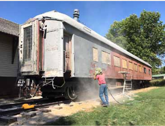
Mobile Blasting Services from Carroll was onsite in late September to sandblast the exterior of the Pullman Car. After repairs, the car was painted Pullman Green.
