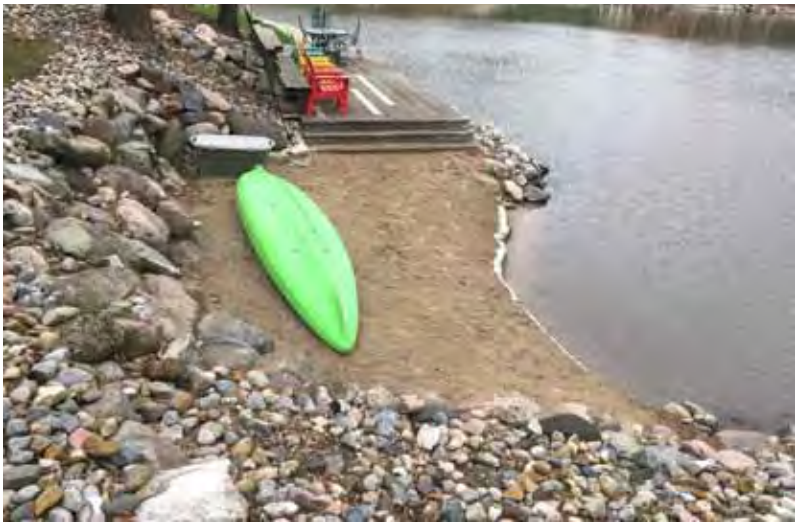
Schlick says lining the wall around the beach with river rock helps slow rainwater runoff.
